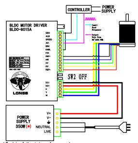
\* The choice of the output power for power supply needs to be made according to the actual condition. Output Power of 350W is just for your reference.
